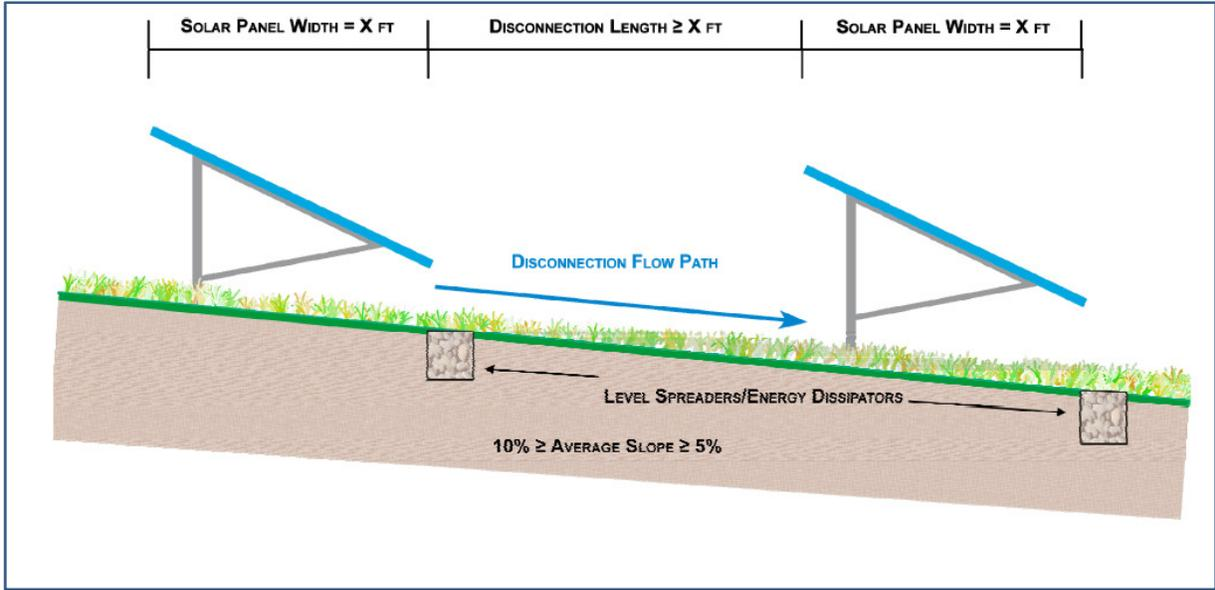
**Fig. 1 Disconnected Impervious Approach for Panels**
