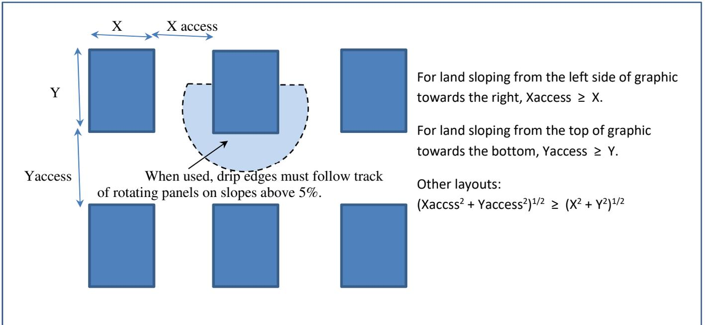
**Fig. 2 Panels on Individual Stands on Slopes**
